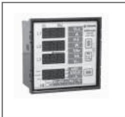
The TEMM-R4-HP is flush mounted DIN 96x96mm with a shallow depth (56mm including terminals). It is an easy-to-use digital multifunction energy meter.
